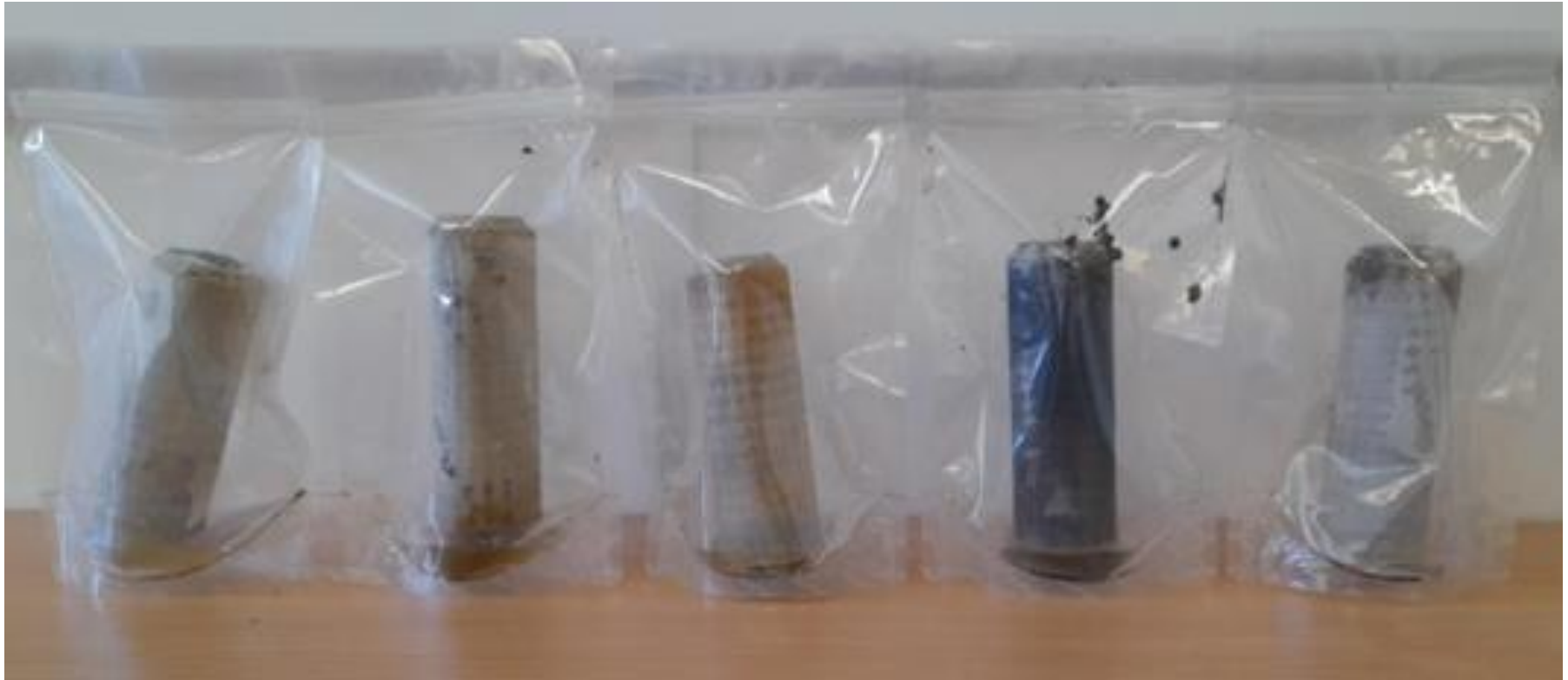
PFAS Flux Meters after 6 weeks in groundwater wells
